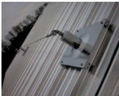
Standing Seam Clamp Fixing Pre Test
